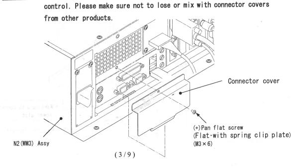
Remove the cap from the version update USB memory stick, make sure that the "CO9" indication is faced up, and insert the memory stick in the USB connector located in the N2 (WM3) Assy.
